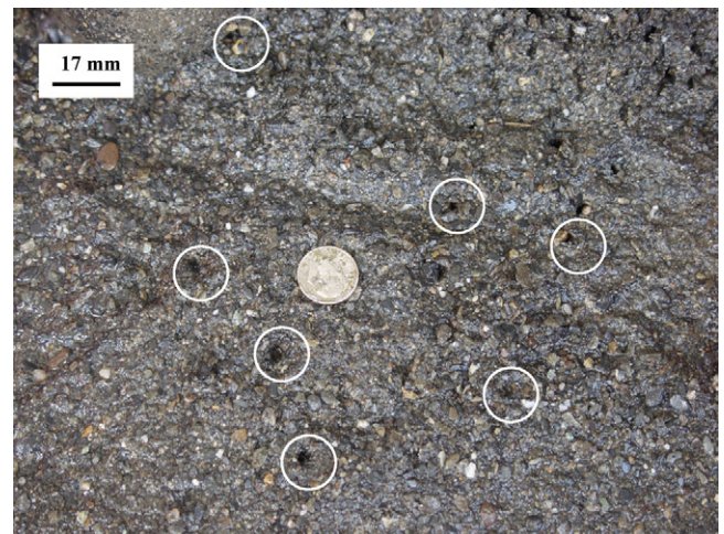
Fig. 4. A top-view of the air-sparging tank showing air-channel exits 120 min of air injection at 80\text{ L/min} (white circles: air-channel exits).
